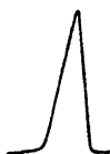
Fig. 3. Gas chromatogram of 2-chloro-2-thio-4-methyl-1,3,2-dioxaphosphorinan made from the corresponding chlorophosphite and sulphur. Column; 5' × 1/8" packed with 20 % PDEAS on 60-80 mesh firebrick. Temperature: 160°C.
